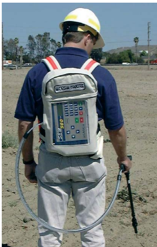
Figure 3: Surface emission monitor being used
